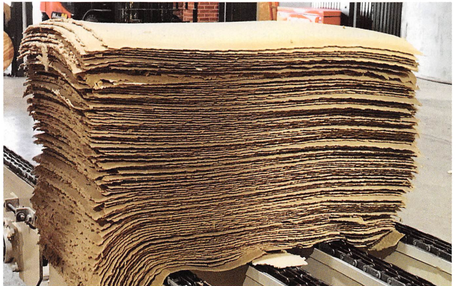
A sample of the wet lap pulp. Moisture content of the wet lap bales will be 50 percent.
